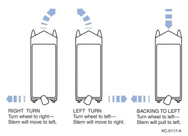
Rotational thrust of the propeller is an aspect most single propeller-driven boats share and needs to be compensated for at slow speeds. During rotational thrust, torque is transmitted to the helm and may cause the boat to drift either port or starboard when moving forward at a slow speed. Rotational thrust usually goes unnoticed at high speeds. While moving forward at a slow speed, constant helm corrections are usually necessary to maintain a straight course.
