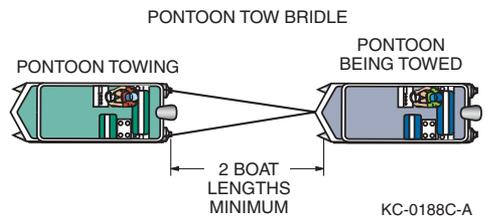
**⚠ WARNING** *Personal Injury Hazard: DO NOT attach tow lines to cleats, watersport line point, or eyes used for docking; use only designated strong points. Death or serious injury could occur if lines and/or hardware fail while they are under extreme tension.*
